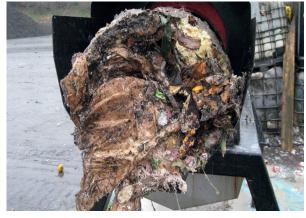
Integrating the RUNI SK370 or SK240 in the processing line reduces the moisture content significantly leading to a weight reduction of the waste of more than 50%\*. At the same time the RUNI extracts extra biopulp from the waste. This ensures a minimization of costs for transportation and incineration as well as a maximization of the output of biopulp.
